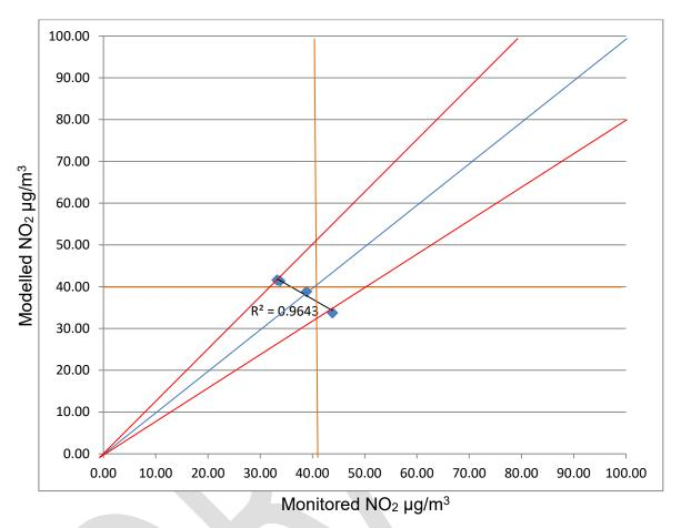
Figure D5.1 NO2 Monitored / Modelled scatter graph
