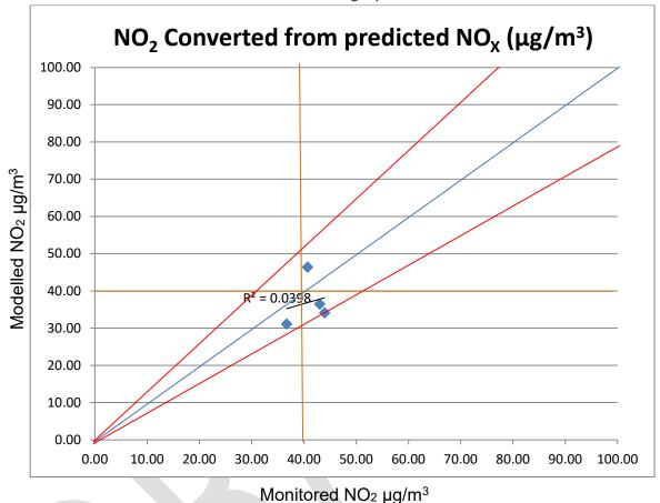
Figure D.3.1 NO2 Monitored / Modelled scatter graph
