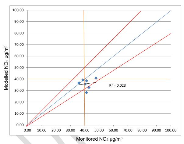
Figure D.8.1 NO2 Monitored / Modelled scatter graph
