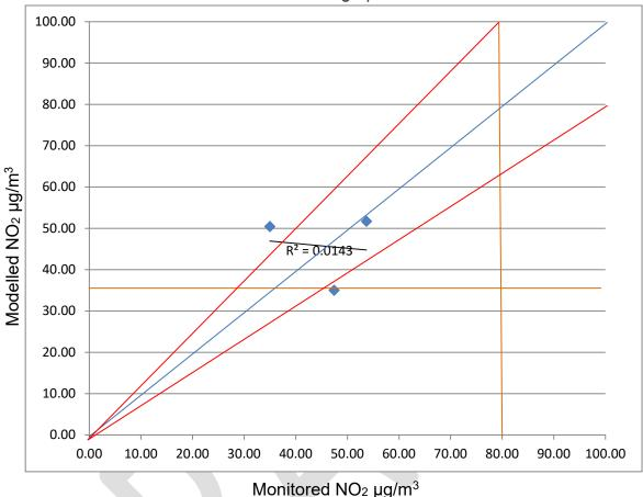
Figure D4.1 NO2 Monitored / Modelled scatter graph
