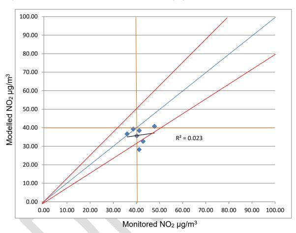
Figure D.6.1 NO2 Monitored / Modelled scatter graph
