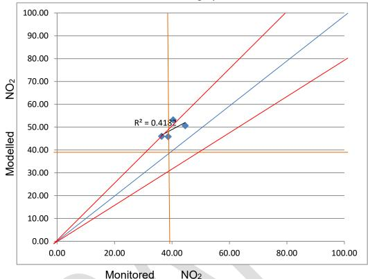
Figure D.2.1 NO2 Monitored / Modelled scatter graph
